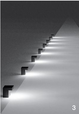
Example 3 The small bollards have a low mounting height of only 8 in. With the source so close to the ground, a distinct bright area is created in the direct vicinity of the luminaire. Luminaire spacing of 8 ft is needed to maintain minimum light levels.
