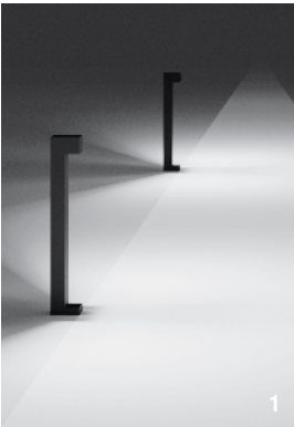
Example 1 The large bollard has a mounting height of 3 ft. The light between fixtures blends together uniformly. The luminaire spacing is 30 ft.
