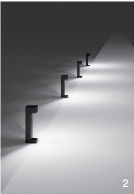
Example 2 The medium-sized bollard has a mounting height of 1.5 ft. The light level variance between fixtures is more noticeable. Here, the luminaire spacing is reduced to 15 ft to maintain the minimum illuminance level.
